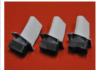
TBC coated HP Turbine blades
